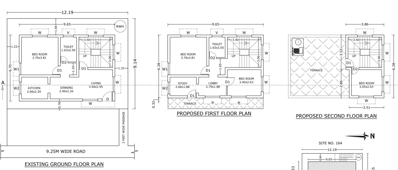
EXISTING GROUND and PROPOSED FIRST and SECOND FLOOR OF A RESIDENTIAL BUILDING EASTERN PORTION OF PROPERTY BEARING NO. 154 GIFTED TO DONEE 9.25 M WIDE ROAD SITE PLAN (SCALE 1:200)
